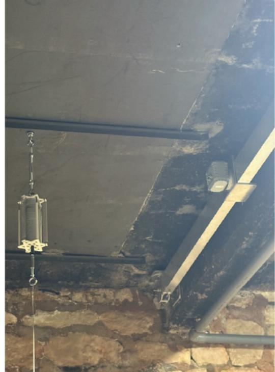
An extensometer was installed between the ground and the floor to measure convergence variations and detect any potential settlement related to the machinery. As a complement, an inclinometer line was installed to precisely monitor deformations of the load-bearing elements, particularly the central beam.
