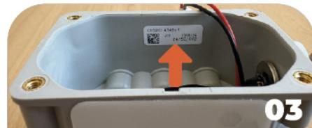
Carefully note the **serial number** (located behind the battery): you will need it to connect the sensor to the application.
