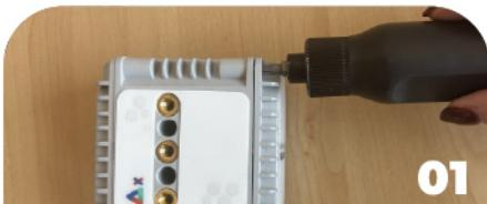
To begin, **remove the DELTA X cover** (2) by unscrewing the 4 screws (7) using a TORX T20 screwdriver.
