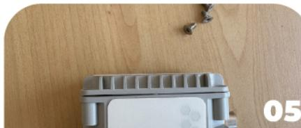
Press on the cover (2) then reinsert the screws (7).
