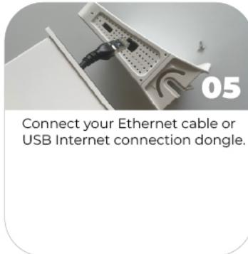
Connect your Ethernet cable or USB Internet connection dongle.
