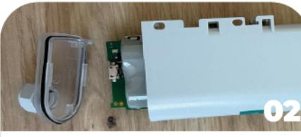
Remove the board in order to connect the USB to USB-B cable.
