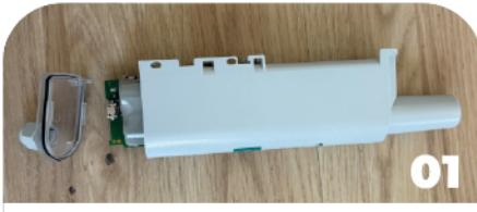
To begin, remove the cover located at the rear of the repeater.
