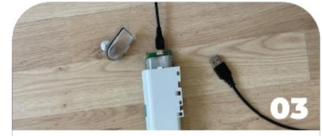
**Use a USB-B data cable** (not a charging-only cable) to ensure proper data transmission.
